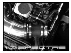
Step 12 Install 4" couplers (with clamps) on both sides of MAFS and install the assembly onto the intake tube as shown (ensure that the arrow is pointing towards the engine). Leave the clamps loose at this time.
