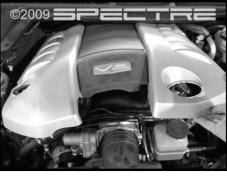
Step 2 Remove the oil cap to allow you to remove the plastic engine cover. Remove the cover and reinstall the oil cap to ensure that nothing falls into the engine while you are working.
