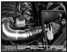
Step 18 Start the vehicle and let it warm up. Shut off and inspect the installation once more for any loose clamps, wires, or hardware. Test drive & enjoy! If you have any difficulties or questions regarding the installation of this intake system, contact the Spectre Performance Technical Department by email - Tech@spectreperformance. com or by phone 1-800-821-4868 Monday thru Friday 6:00am to 4:30pm PST.
