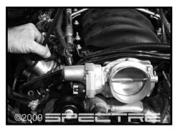
Step 8 Disconnect breather hose from Step 4 on the engine side. This will be replaced later with a new hose from the kit.
