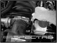
Step 3 Once the engine cover is removed, loosen the clamp on the stock air intake around the throttle body.
