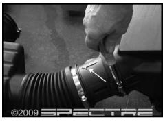
Step 10 Remove Mass Air Flow Sensor (MAFS) from the stock intake system. Note the arrow on the sensor indicating the direction of flow. The arrow must ALWAYS point towards the engine when installed on the vehicle.
